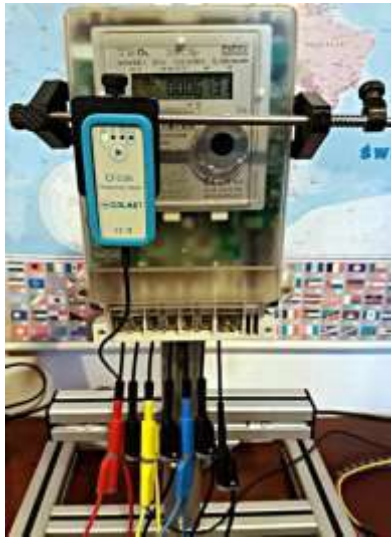
Connected meter ready for testing
