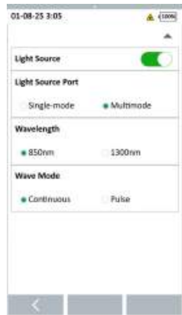
Multimode Light Source is enabled. Connect to the TX port on the right as indicated on the screen.
