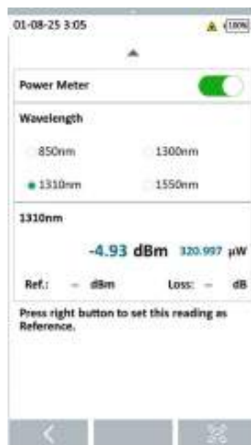
Power Meter is enabled. Connect to the RX port in the middle as indicated on the screen.
