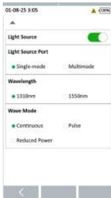
Single-mode Light Source is enabled. Connect to the TX port on the left as indicated on the screen.
