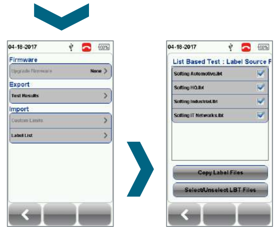
Importing Label Lists into WireXpert via USB stick
