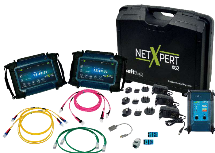
Figure 2 - NetXpert YG2plus with two main devices for fiber qualification and one active remote for copper qualification
