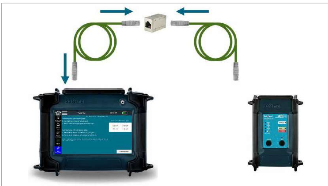
Figure 39 - Test setup for setting the reference - Cu
