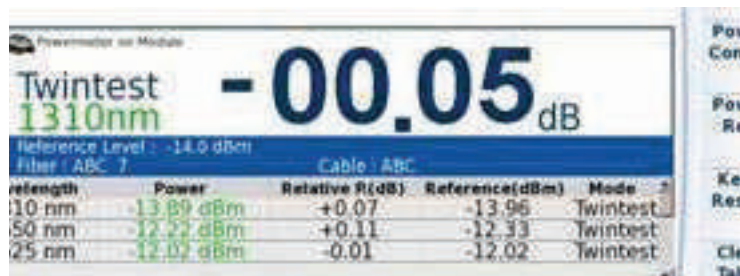
Fig. 48 Results and commands of the power meter
