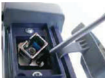
Fig. 17 Fixing the adapter
