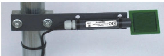
Typical Mounting of the Leaf Wetness Smart Sensor
