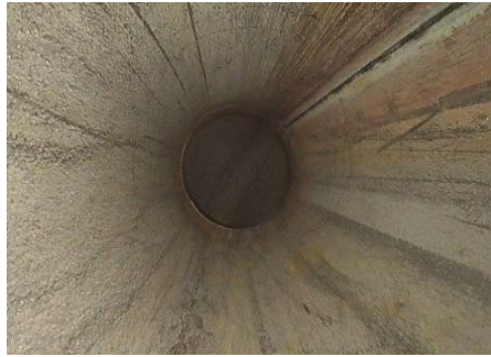
6.0mm Probe with centering device Better light distribution & overall view of the inspection environment
