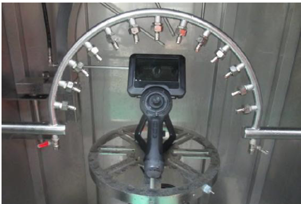
X750 Probe under dust and water proof test
