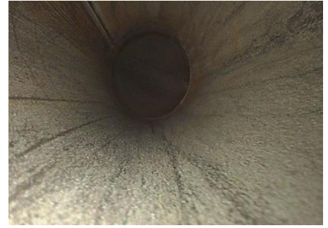
6.0mm Probe without centering device Lack of light distribution & missing the upper view of the inspected environment
