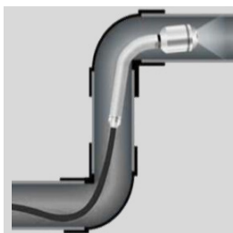
Capable of passing through two 90° pipeline turns
