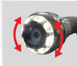
Mechanical self leveling camera tip
