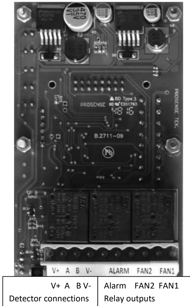
Diagram 9: Control panel zone module board
